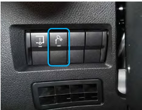
Work lamp switch on the instrument panel
