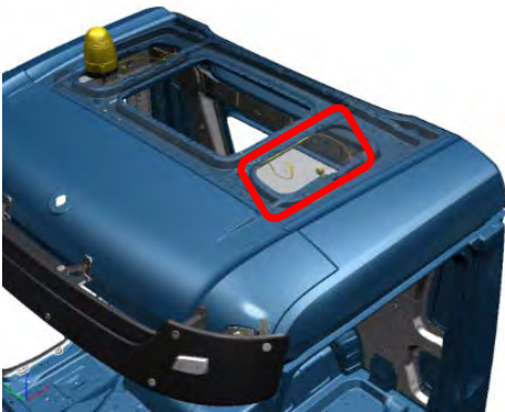
Installation location of electrical connector X1.1 in the area above the driver's seat (S, M and L cab)
